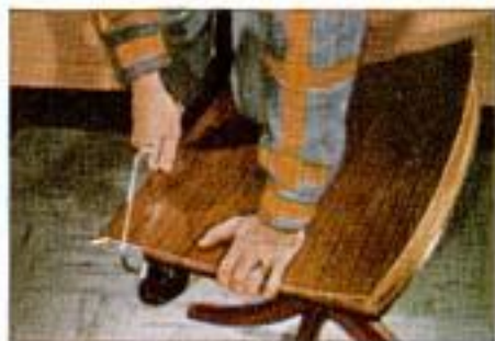
3. Saw Formica top side up with fine tooth saw.
